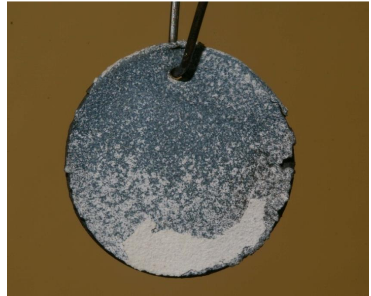
Valve steel sample oxidized in cyclic conditions
